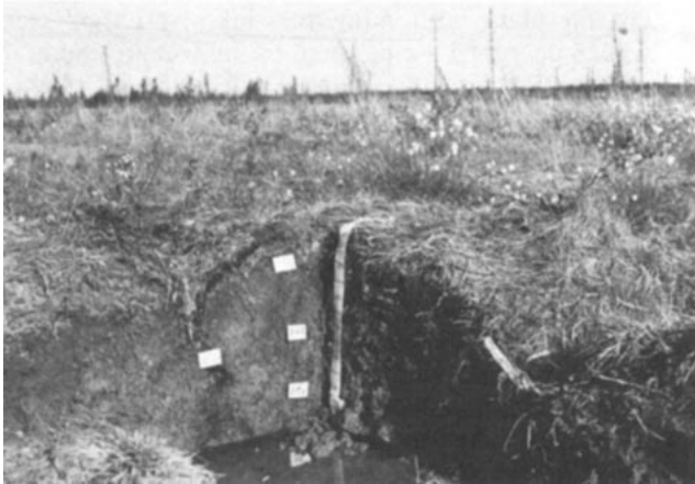
Fig. 3. Minimum of Brunlsolic Cryosol or Pergelic Ruptic Cryaquept showing involuted organic matter, Omy, in trough between hummocks. (Slide 4)
