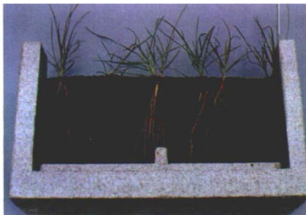
Fig. 2. Rhizotron with cover removed to expose root systems.
