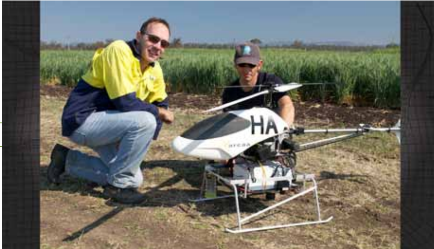
Researchers at CSIRO use a remote-controlled gas-powered model helicopter called the “phenocopter” to measure plant height, canopy cover, lodging, and temperature throughout a day. Pictured here are Scott Chapman (left), a principal research scientist at CSIRO, and Torsten Merz, developer of the phenocopter.
